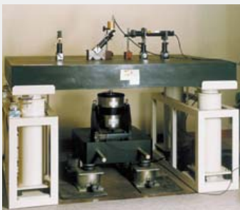
Absolute calibration setup for vibration accelerometers
